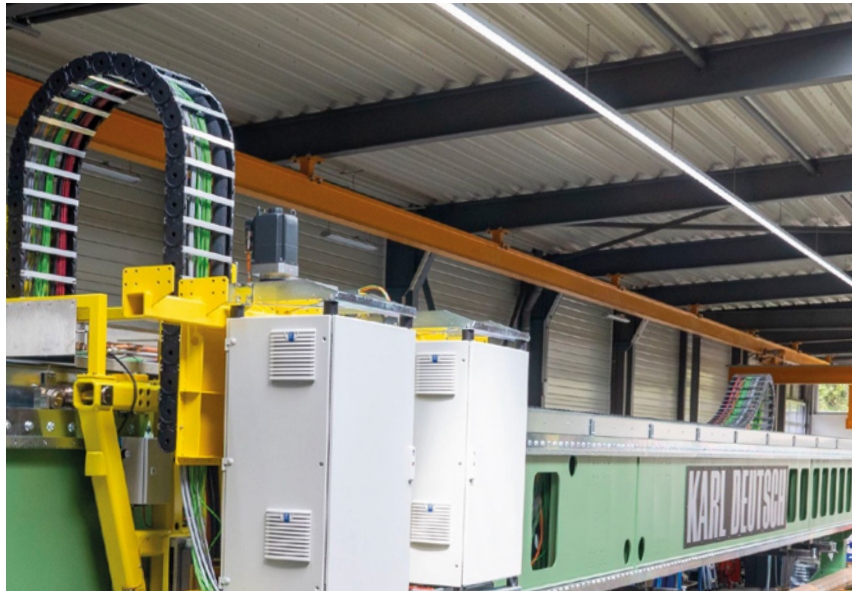
The customised energy chain system facilitates accurate measurements and reliable functionality of the testing system.
