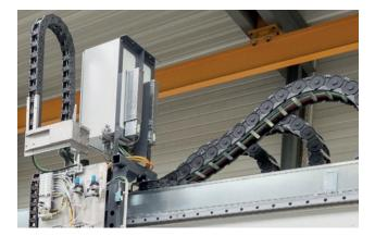
EKD Systems GmbH has specialised in drag chain systems made of plastic, steel, aluminium and stainless steel for more than 50 years. The portfolio includes open, closed and partially closed drag chains for gliding and self-supporting applications.
